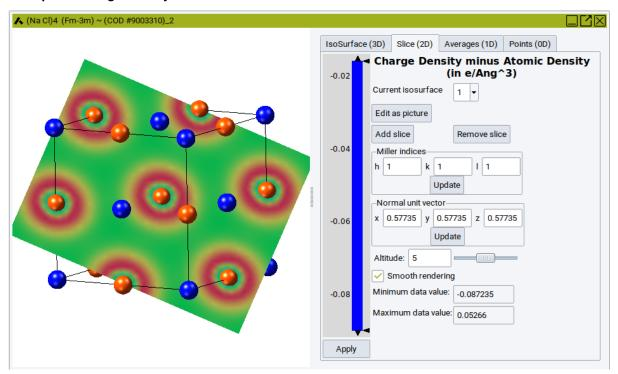
In the above example, a projection of the difference charge density onto the (111) plane is shown for NaCl. The range of the plot is from -0.087235  $e\mathring{A}3$  to 0.5266  $e\mathring{A}3$ . The plot has three sections: The lowest section ranging from -0.09 to -0.016 is colored in blue. The section from -0.016 to 0.035 shows the variation of the
